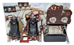
The coil block assembly appears not original, the 6.3V transformer was mounted differently, and proper valve sockets were used in this variation. This \*might\* lead to the believe to be a post war replica if not for an original Kongshavn double tuning capacitor was used.
