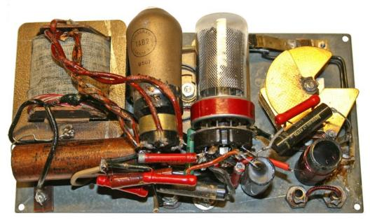
Internal view of Kongshavn variation 1. The valves were an ECH21 regenerative detector/AF amplifier and a TAB2 HT rectifier. Note the ubiquitous double tuning capacitor.
