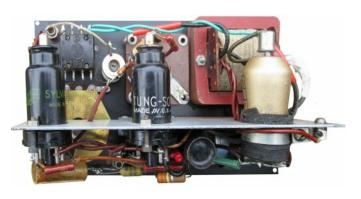
Front panel and internal view of Kongshavn variation 3. As there were no valve sockets available at the time, the valves were just wired into the circuit. Note that several components and part of the original wiring had been replaced at a much later stage.
