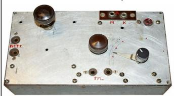
A recently found Kongshavn variation 4 employed a 6K7 and 6F5. There was no rectifier and an external +HT source should be connected to the red marked banana type socket located on the top right of the front panel.
